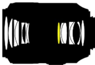
Figure 4: Optical construction of the AF-S Micro-Nikkor 105 mm f/2.8G ED; yellow: Lens made of ED glass. (image source: Nikon sales brochure).
